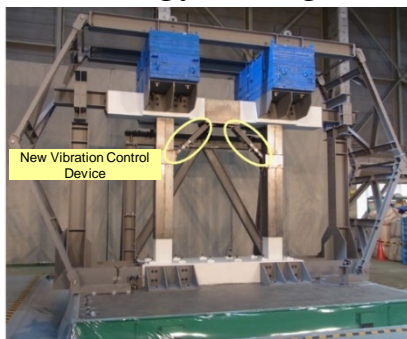
Elevated bridge displacement suppression control with new vibration control device (earthquake countermeasures)
