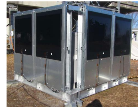
Noise-blocking walls with perovskite solar cells, under demonstration testing
