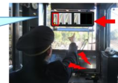
Image of detection by a safety confirmation support device that uses image recognition technology
