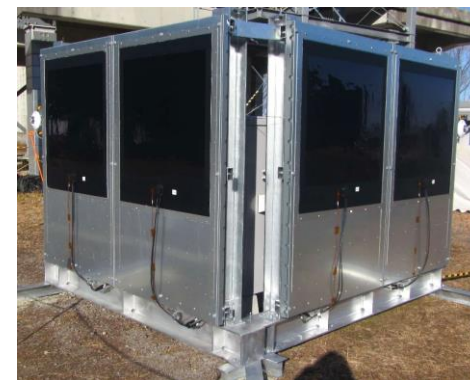
Noise-blocking walls with perovskite solar cells, under demonstration testing
