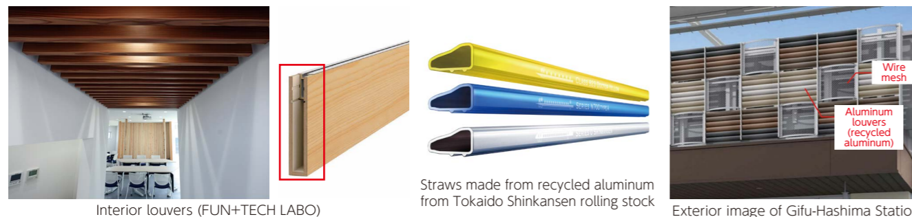
Manufacturing process and usage examples (metal bats and station building) of recycled aluminum from Tokaido Shinkansen rolling stock * Images in ② and ④ courtesy of SUS Corporation, and image of bats, of Mizuno Corporation
