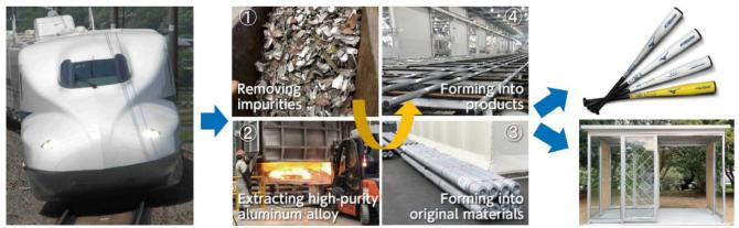
Manufacturing process and usage examples (metal bats and station building) of recycled aluminum from Tokaido Shinkansen rolling stock \* Images in ② and ④ courtesy of SUS Corporation, and image of bats, of Mizuno Corporation
