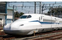
The N700S is the first high-speed train equipped with a battery-based self-propelled system. It can travel to a location
