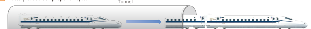
The N700S is the first high-speed train equipped with a battery-based self-propelled system. It can travel to a location where passengers can safely evacuate in the event of a long power outage following a natural disaster, etc.
