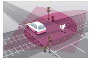
High-performance crossing obstacle detection system (laser sensor type)
