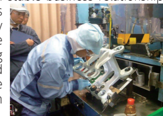
Conducting a quality audit of rolling stock components
