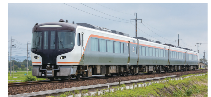
Hybrid-powered limited express rolling stock, Series HC85
