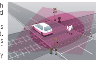
High-performance crossing obstacle detection system (laser sensor type)
