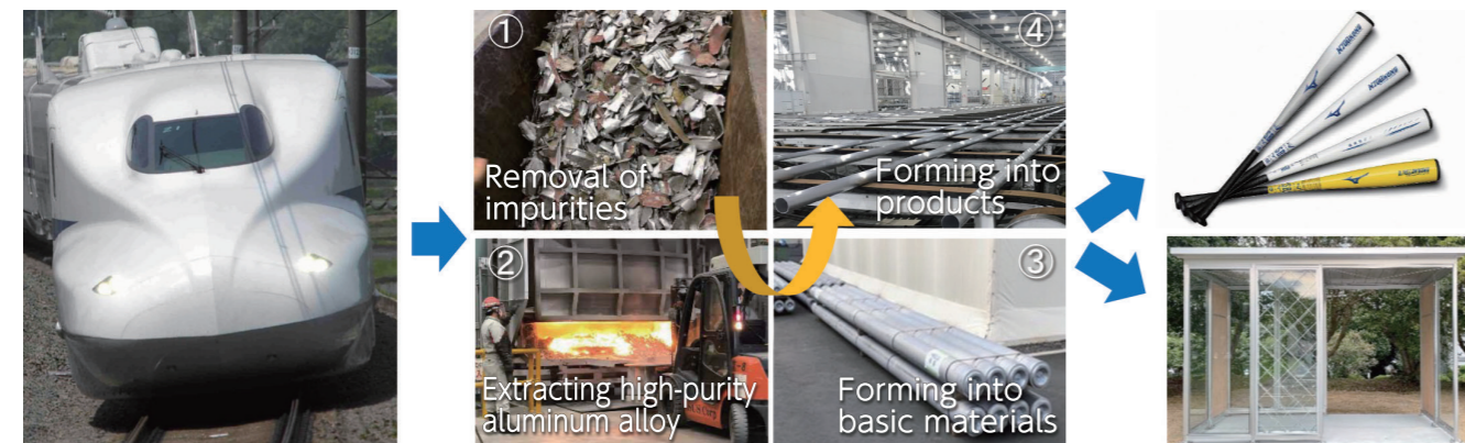
Manufacturing process and usage examples (metal bats and station building) of Recycled aluminum from Tokaido Shinkansen rolling stock *Images in ② and ④ courtesy of SUS Corporation, and image of bats, of Mizuno Corporation
