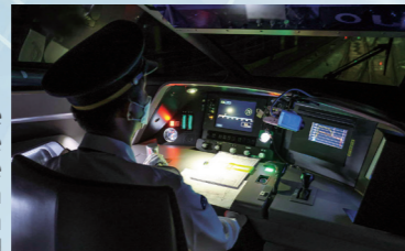
Aiming for the commercial introduction of trains equipped with automated train operation functions* of the automated train operation system (GoA2) around 2028, we are currently conducting running tests. * Scheduled operation functions, fixed-position stopping functions, etc.
