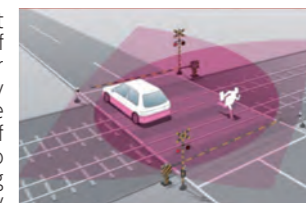
High-performance crossing obstacle detection system (laser sensor type)
